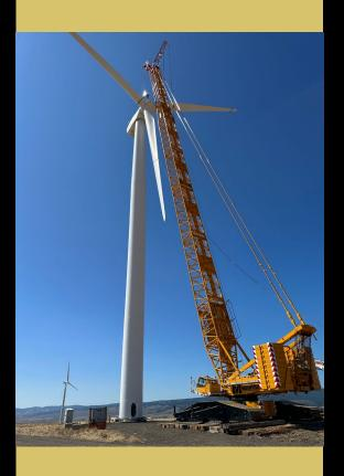
For Rent! The LR 1600 is designed to handle heavy lifting tasks with its impressive lifting capacity. Its load capacity can vary depending on the configuration and additional equipment, but it is generally capable of lifting loads in the range of 600 to 800 metric tons.
