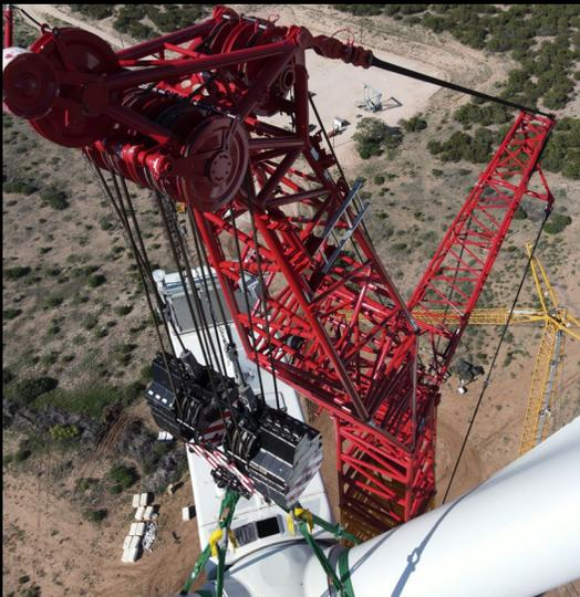
A Titan in the crane industry, the Liebherr LR 11000 has proven to be an invaluable tool in our fleet. The LR 11000 has an impressive max hoist height of 220 meters, a max load capacity of 1,000 tons and a max radius of 184 meters. These abilities and its dynamic versatility have made it an instrumental tool for several of our wind maintenance projects. Recently, one of our wind O&M clients came to us with a challenge. They needed to remove a damaged wind turbine rotor.
