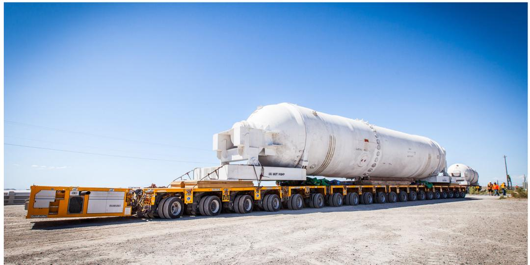
Mountain Heavy Transport participated in the largest ever pick and transport at Energy Solutions in Clive, UT. The piece was a 1.2 million pound steam generator that was offloaded from rail, transported to a containment cell, and set on to sand saddles. We utilized a 700 ton gantry and 20 lines of Goldhofer SPMT for the project. The job involved months of planning and ultimately a lot of hard work.
