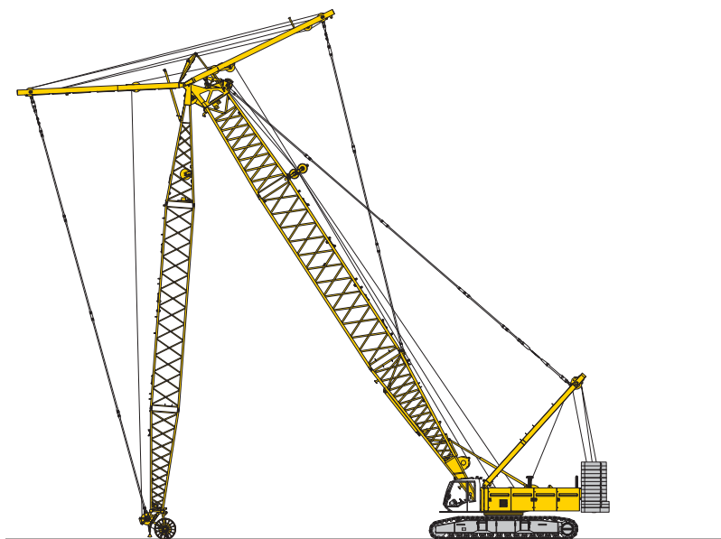
Erecting of main boom and luffing jib
