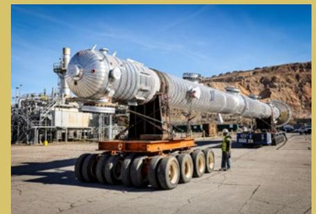
on the vessel during transport. The vessel was delivered to 600 ton and 350-ton hydraulic cranes for standing and final set to foundation. The transport, although short, was highly technical and involved extensive planning and was executed flawlessly.
