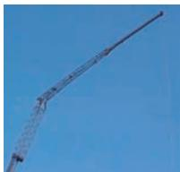
A bi-fold swingaway lattice extension easily stows on the side of the base boom for easy transport. The choice of a manual or optional hydraulically offsettable extension is available. To take
