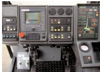
Crane functions are controlled by ECOS (Electronic Crane Operating System) with CAN-BUS. The EKS4 load moment indicator provides detailed feedback and control of the cranes operating functions. Electronically controlled ISM 450 diesel engine delivers plenty of power on and off the jobsite.
