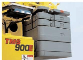
Up to 31,500 lbs of counterweight can be power installed and removed from the superstructure cab, making transporting a breeze.
