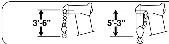
**DIMENSIONS ARE FOR LARGEST GROVE FURNISHED HOOK BLOCK AND HEADACHE BALL, WITH ANTI-TWO BLOCK ACTIVATED.**
