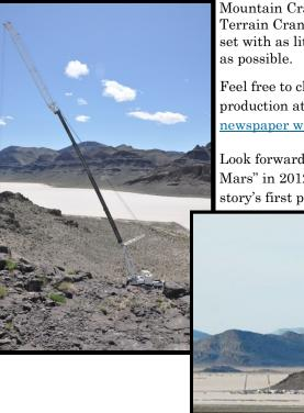
Mountain Crane's 500 Ton Demag AC1300 All Terrain Crane was utilized to place equipment on set with as little of an impact to the environment as possible.
